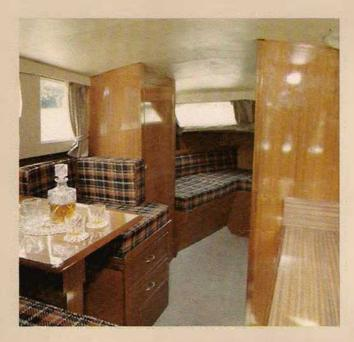
In the main cabin the dinette is to port and the galley to starboard, the galley is fitted with a grill and two burners, gas is supplied from a bottle stowed in a metal container, vented to the outside, fitted against the transom, a good size sink with water pump, the whole galley area has a double hinged top so when not in use the area can be closed and used as a sideboard, four stowage lockers provide ample space for food and utensils.
