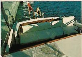
THE COCKPIT offers a large rear seat which can also be used as a fifth berth, and from the helm there is good all round vision. Water tanks hold 60 gallons, whilst fuel is 35 gallons per engine. There is a good range of upholstery and carpet alternatives and white curtains are hung as standard.
