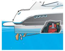
impeller pump mechanically driven from the engine. The cooling water eventually exits via the water cooled exhaust. When the engine is running it is important to monitor water flow through the exhaust outlet.
