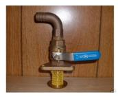
on the engine intake. Craft fitted with sea toilets generally have inlet and outlet valves as well. Some insurance companies insist gate valves are closed when the craft is unattended, so check your policy. Remember to turn on cocks before starting the craft. Labels on the dashboard are the best reminder.
