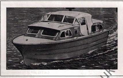
The centre cockpit version of the Elysian 27 is an alternative to the highly successful aft cockpit model, the raised centre cockpit giving excellent all round viewing.
