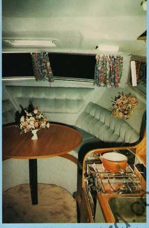
Cabin access is to starboard down two carpeted steps, there is an abundant use of teak carpentry, with walls and ceilings lined in foam-backed blue/grey vinyl and hessian, which compliments the richness of the wood.
