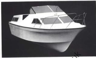
The VIKING 800 is a six-berth centre-cockpit offshore cruises giving spacious accomedation in two private separate cabins, both with full standing headroom. Suitable for single or twin inboard engines.
